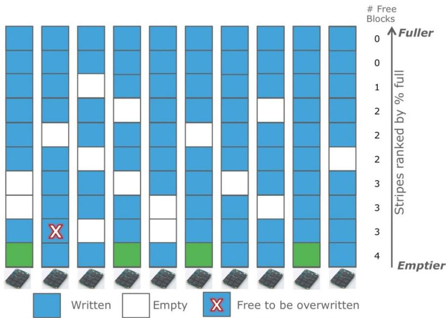
Figure 9: XDP always writes new data into the stripe with the emptiest space (the one at the bottom of the stack). In this example, four blocks were free (two were empty and two were available to be overwritten). Through this method, XDP amortizes the stripe update I/O overhead as efficiently as possible.
