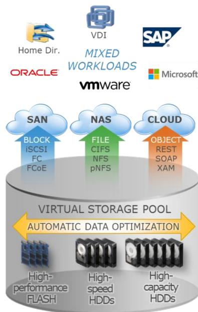
Ideal for mixed workloads, both physical and virtual, The VNX family next-generation storage platform is powered by the latest Intel Multi-Core Xeon E5-2600 series with a 6-Gb/s SAS drive back-end and delivers more firepower, greater efficiency, better protection – all with ease.
