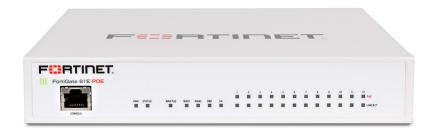
The FortiGate 80E series provides an application-centric, scalable and secure SD-WAN solution in a compact fanless desktop form factor for enterprise branch offices and mid-sized businesses. Protects against cyber threats with system-on-a-chip acceleration and industry-leading secure SD-WAN in a simple, affordable, and easy to deploy solution. Fortinet's Security-Driven Networking approach provides tight integration of the network to the new generation of security.
