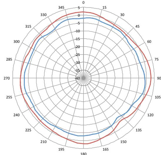
— 5.5GHz Average Azimuth — 5.5GHz Average Downtilt 30
