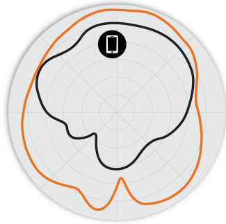
Figure 3. H350 5GHz Azimuth Antenna Patterns
