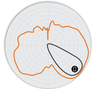
Figure 7. R560 6GHz Elevation Antenna Pattern
