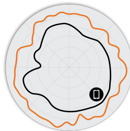
Figure 3. R760 5GHz Azimuth Antenna Patterns
