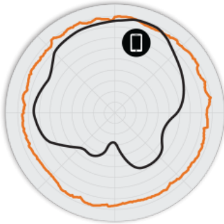
Figure 2. R750 2.4GHz AzimuthAntenna Patterns
